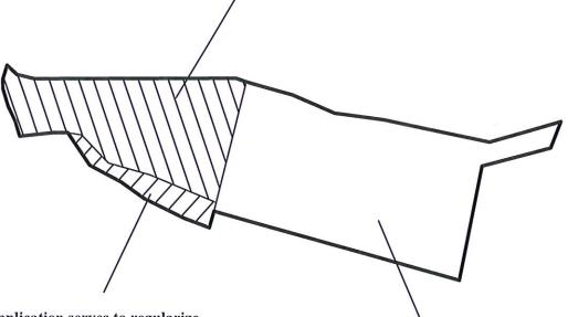
This application serves to regularize the existing filling of land with concrete of this portion of site (about 101m²) of about 1.5m in depth to provide a solid ground for erection of structures and vehicle maneuvering
